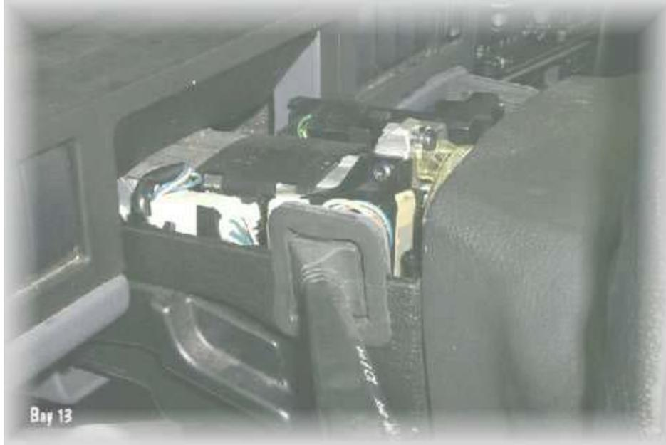
Once you have worked the top off, slide the column lock open and work the bottom plastic cover off, it fits snug over the key side of the ignition.
