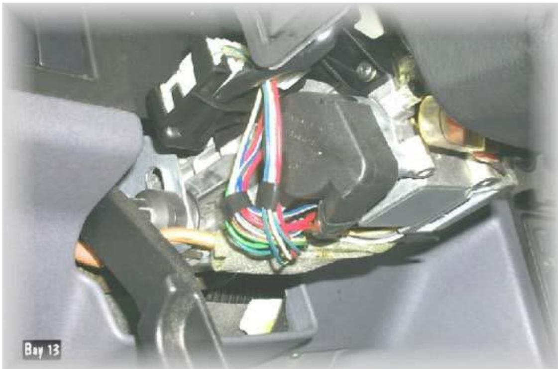
Once the bottom is off and the steering lock down and the column pulled out all the way, you will have a nice view of the connector that goes on the switch. The connector just pulls off the switch do it carefully, there are 8 pins on the switch and the connector cover could come off in your hand.
