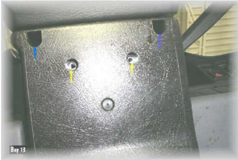
Drop the steering wheel down and pull it back. You will need a 15 torx and a 25 torx to get the bottom plastic cover off the steering column. What I use is a 15 torx that I picked up at Sears because it is about 8 inches long and can reach up into the small holes that the blue arrows are pointing too. The yellow arrows are where the 25 torx screws go. Once the screws are off the bottom you can remove the top half.
